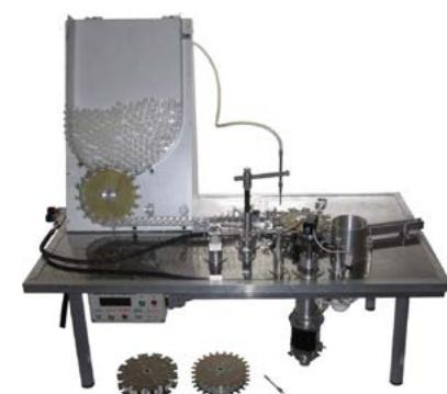
Equipment for filling and sealing glass ampoules
