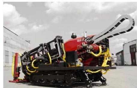
*tension-wire pipe destroyer PUNCHER CRASH 60*
