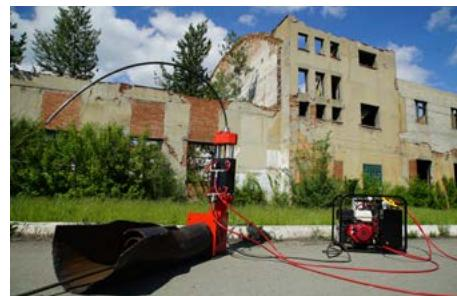
*Plant for controlled soil puncture for wells PUNCHER 20CS*
